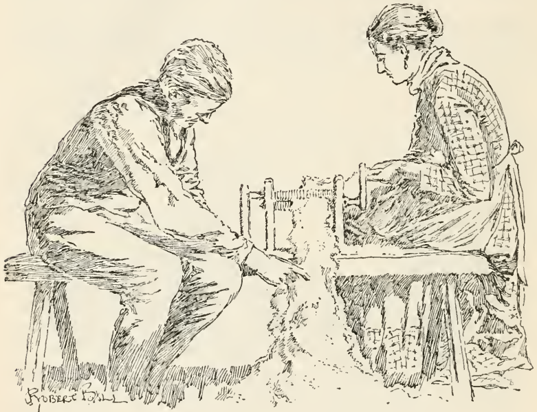
A COTTON GIN, A SIMPLE MACHINE FOR SEPARATING THE SEEDS FROM THE COTTON, INVENTED BY ELI WHITNEY
